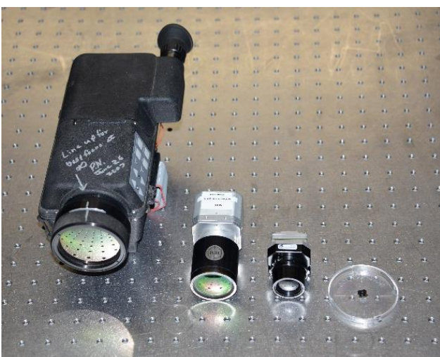
Fig. 1.3 Uncooled thermal infrared imagers used in our lab since 2001. The current study uses the tiny imaging module sitting in a plastic dish on the right-hand side.
