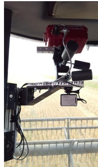
Fig. 1.1 Custom and off-the-shelf cameras mounted in a combine during harvest.
