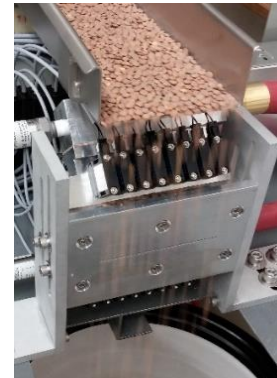
Figure 2.6 Waterfall sorting testbed.
